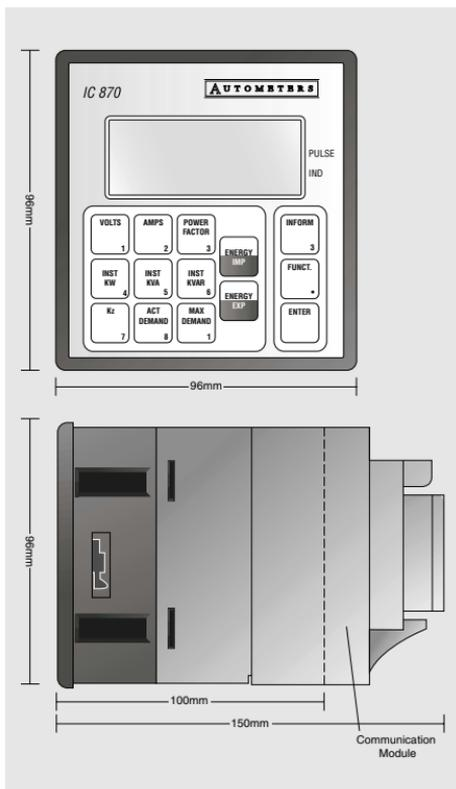
Figure 1. Installation details
